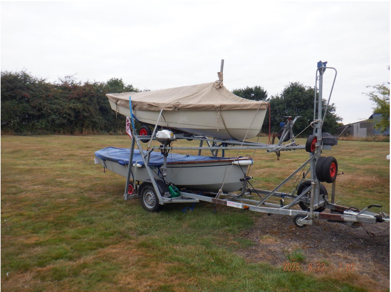
Linling over Essling on West Mersea designed and built double stacking trailer owned by PTK towed by Yvonne Mitchell (by PTK)
