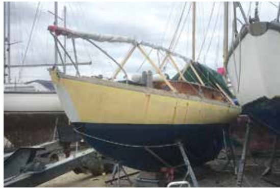
Storm damage repaired. All ready for new rubbing strakes.
