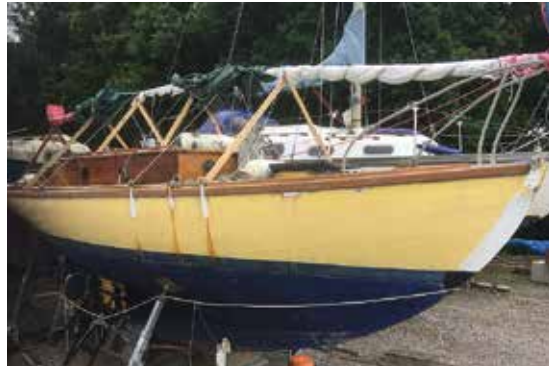
New rubbing strakes all secured prior to varnishing. Several coats of epoxy have been applied underneath.
