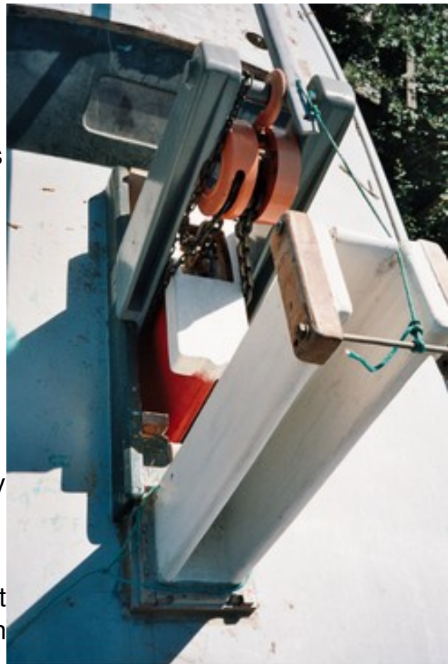
Tabernacle and keel lifting arrangement
