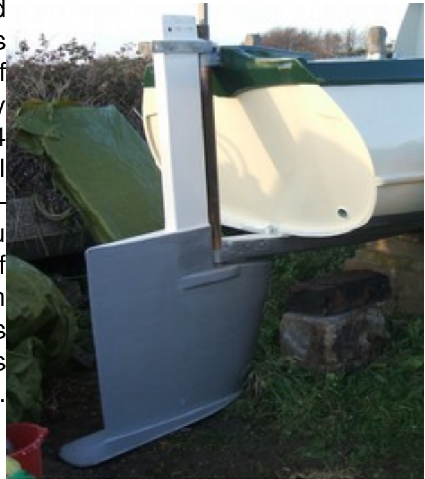
The rudder..... note skeg, tube for pintle, bottom end plate . The bumpkin is set in the aft end of the upper rudder gudgeon
