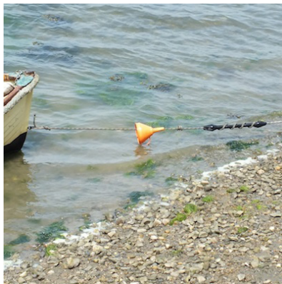
Step 1: The line is set on the stem. Note the funnel needs to be close to the stem so when the tow line goes slack and the dinghy runs on, it deploys as a drogue quickly.
