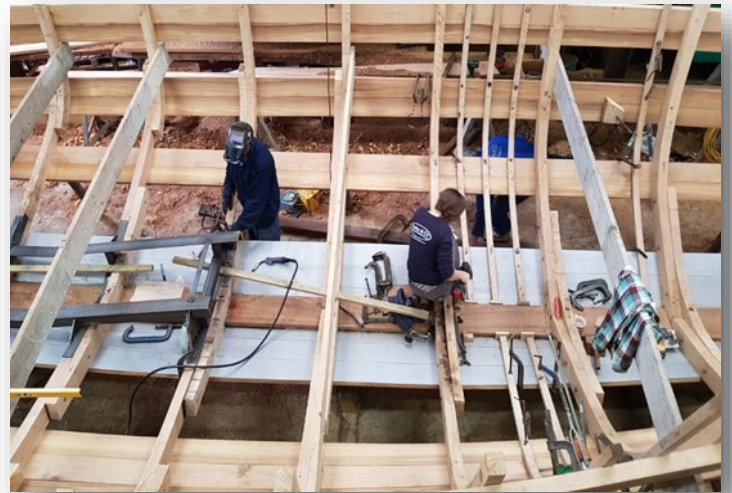
James welding the engine beds, Holy and Graham fit the ribs
