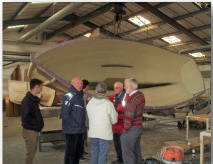
Hull being rotated to finish gel coating
