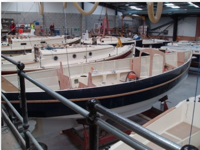
Hulls being fitted out before the deck & cabin roof are fitted
