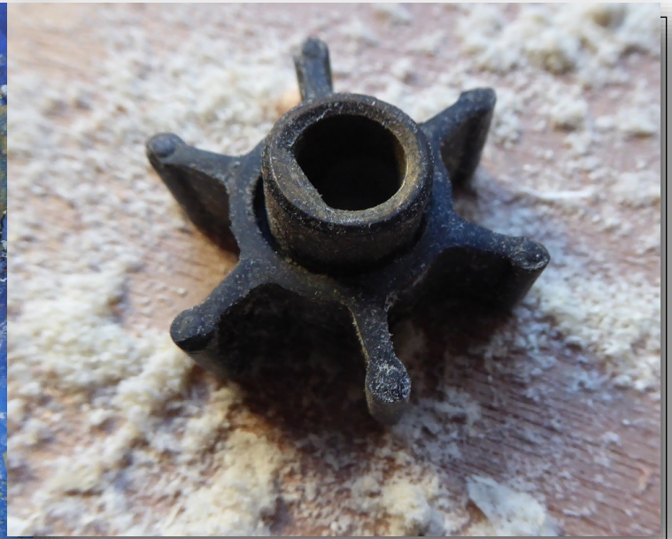
The unequivocal death of an impeller
