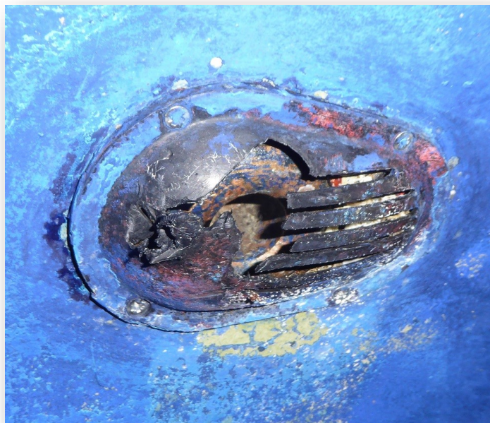
Knifed grid after concentrated pressure washing to remove the anti-foul mask and expose it properly back at the boatyard.
