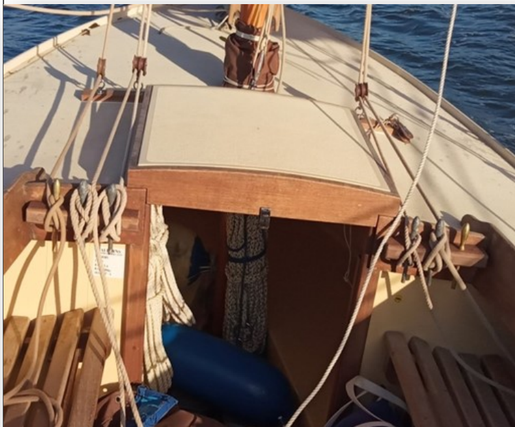
New three pin rails glued and with long screws and new turning blocks
