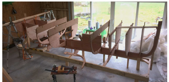
Backbone, Bulkheads and Frames (Photo Nick Fox)
