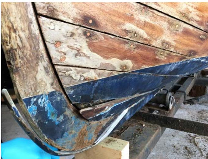
*Planking and Stem repairs required*
