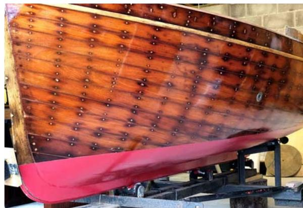
*Hull repaired re-caulked and finished*
